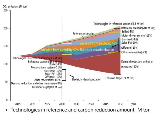
1.The amount of carbon reduction from electricity use(motor-driven system and low carbon power contribution) is much greater than the carbon reduction of fuel combustion emissions (boiler contribution)
